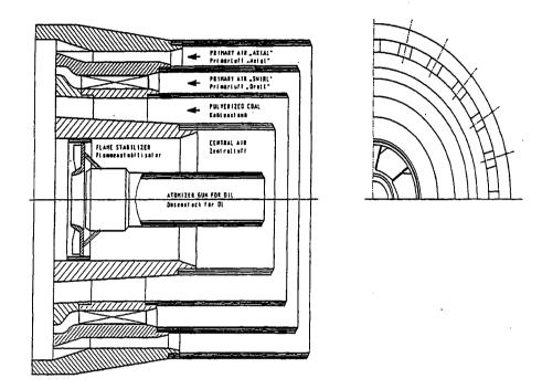
The particular feature of the KHD Pyrojet Burner (Fig. 5) is the jet air. The effect of this burner can be explained by the better and more uniform mixing of fuel and secondary air due to the jet air being introduced at nearly sonic velocity. For this reason the Pyrojet requires a compressor for the jet air.
